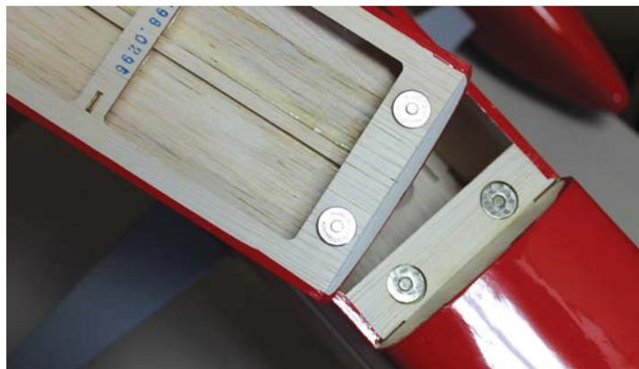
(above right) fasten the rear of the top tank/battery hatch. Pins secure it from the front. Larry found it very handy, even with a glow-powered plane, to be able to instantly check the remaining fuel level.
