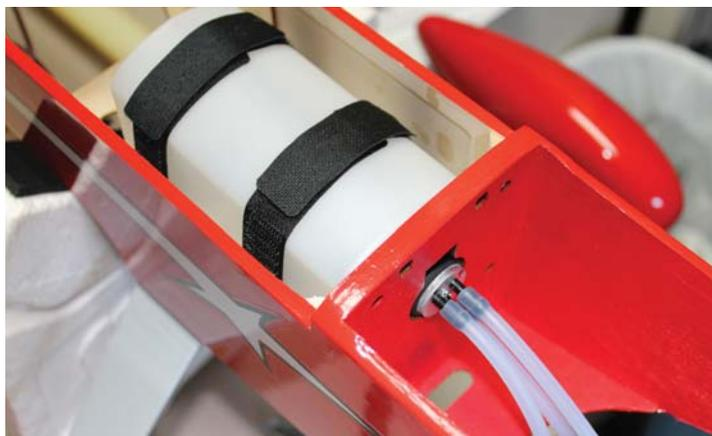
The tank is held in place with hook-and-loop straps. The fuel lines run through a pre-cut hole in the firewall (above left) for the tank stopper. When fully mounted, a small supplied balsa block will be glued at the back of the tank to keep it from sliding backward, and a specially cut tank bracket will be glued in place mid-way between the straps to keep it centered in the compartment. The
