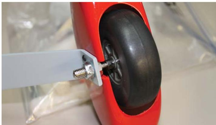
The landing gear components received high marks from Larry for their sturdiness and fit. The wheels (above left) are a dense foam that seem to wear well and at the same time provide some landing cushion. Paired magnets
