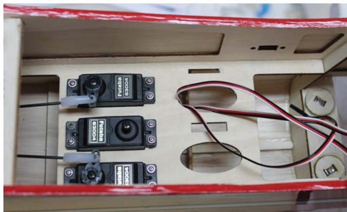
roomy fuselage interior (above right) provides lots of room for installing all components as well as having handy cut-outs for whichever type of power selected. Note the standard receiver switch cut-out on the far fuselage wall. The near wall contains a larger cut out for switches with integral charging jacks. The circles at the right are mounting supports for the hatch magnets.
